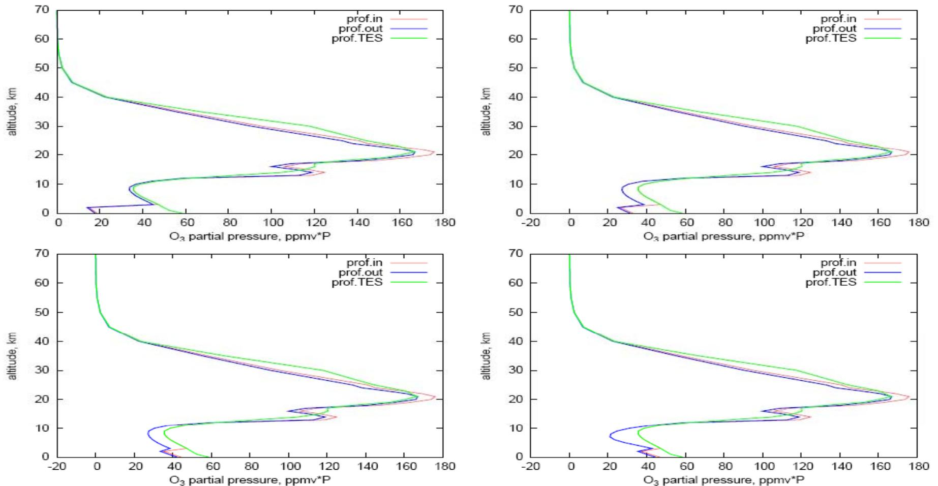
Figure 3: The retrieved ozone atmospheric profiles for the 23<sup>rd</sup> of April 2007, 09h22m and 11h15m (upper figures) local time, and 14h35m and 15h40m (lower figures) local time. On this day the values of both total ozone columns (411.0 DU by FTIR) and tropospheric ozone columns are very high. Possibly we are here observing a stratospheric intrusion event as the highest OMI value of total ozone column in 2007 was 448 DU for the 22<sup>nd</sup> of April 2007.
