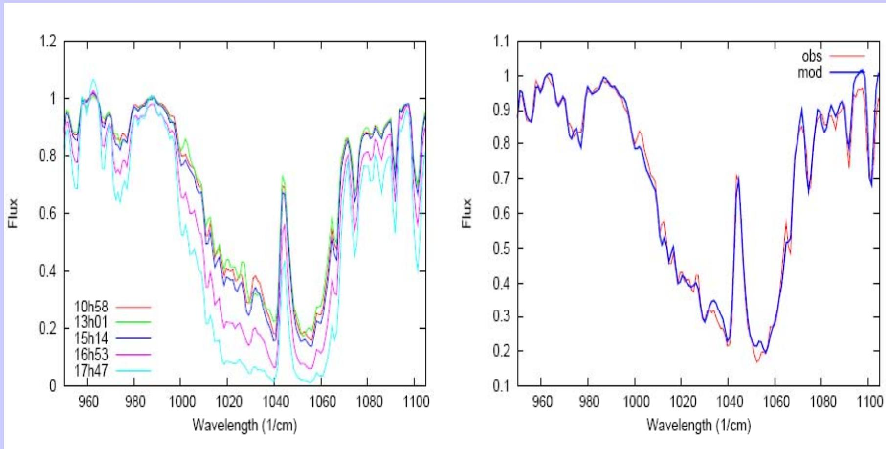
Figure 2: The observed FTIR spectra of the 9.6 micron ozone band for the 29<sup>th</sup> of September 2007 (29.09.07) (left) and the comparison of the observed FTIR spectra and modeled MODTRAN 4 spectra following the procedure for best fitting for the observation at 13h 01m local time on this day.
