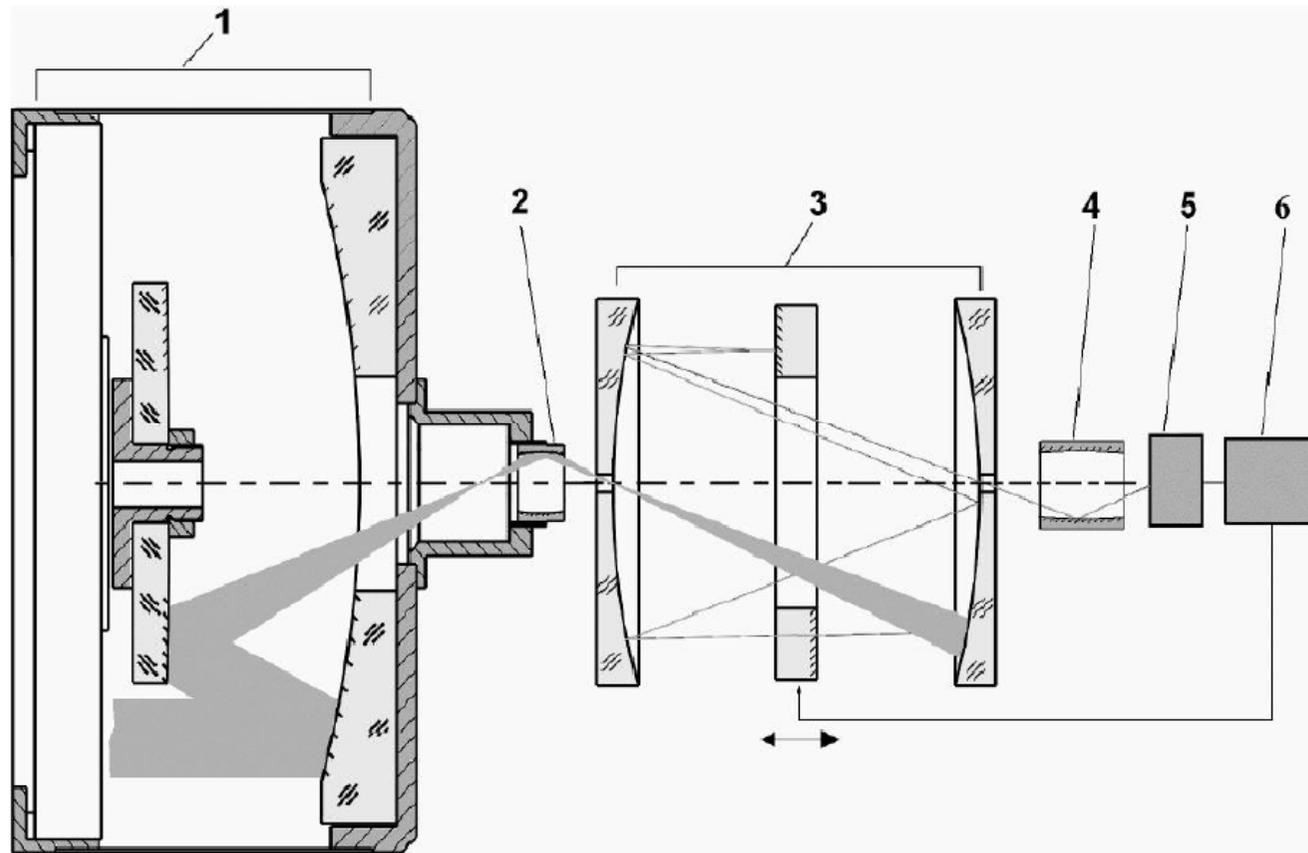
**Figure 1.** Structural and optical scheme of the FTIR spectrometer : 1 - fast lens; 2, 4 - ellipsoids for shift of image; 3 - interferometer ; 5 - detector; 6 - electronics block.
