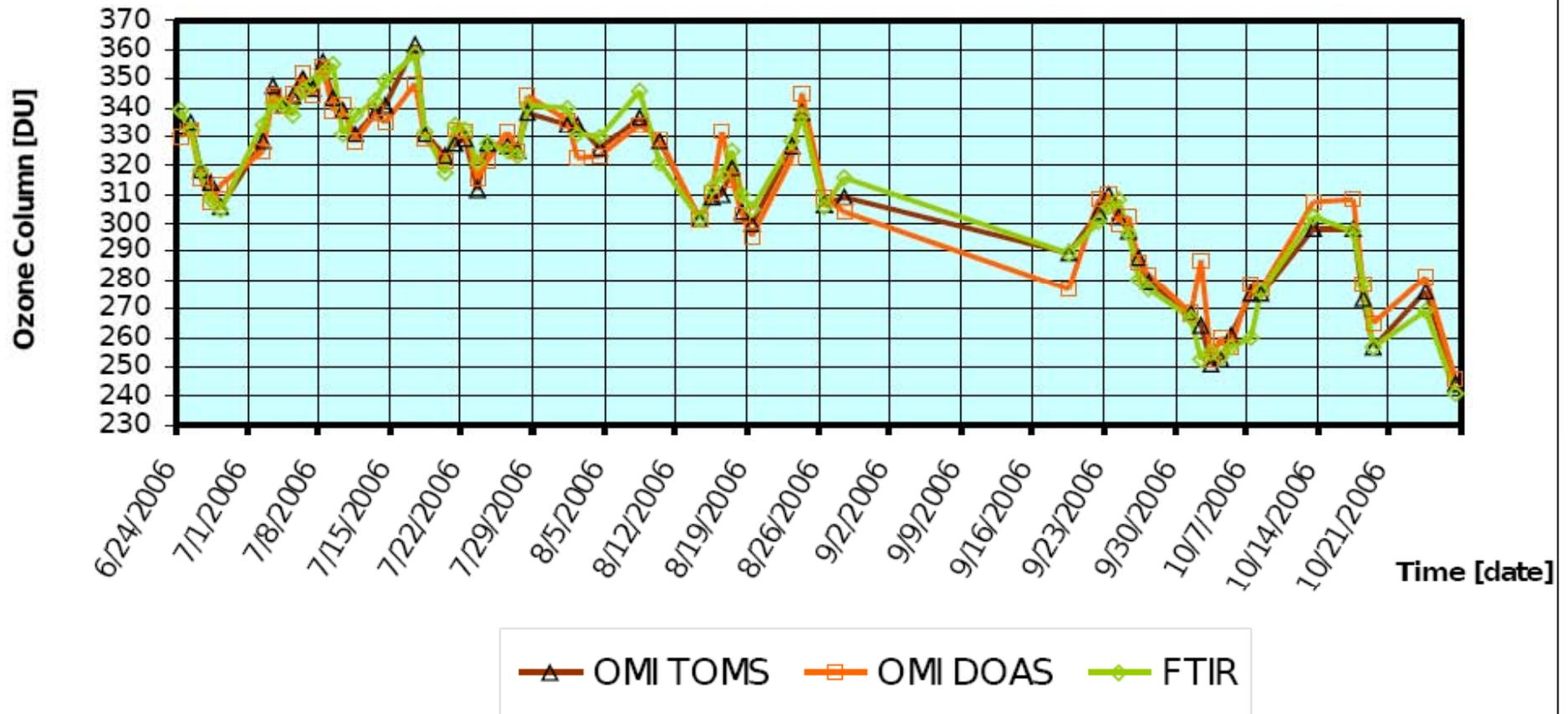
Figure 1: Time series of the OMI total ozone column and the ground based FTIR total ozone data of 2006 for the ground site of Kiev (MAO). Average difference of satellite minus ground based amounts to 0.37 DU and -0.25 DU for OMI-DOAS and OMI-TOMS respectively, with a 8.77 DU and 5.37 DU standard deviation (1.11 DU and 0.68 DU standard errors).
