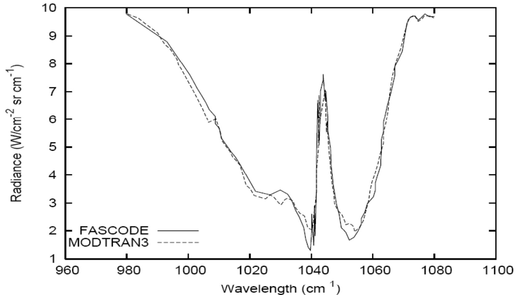
**Figure 3.** Comparison of MODTRAN (Band Model) and FASCODE (line-by-line) spectral radiance calculation for ozone 9.6 micron band (from *Bernstein et al.* [1996]). We estimate the value of the sample variance of these two spectra fit in the range of 981 – 1078
