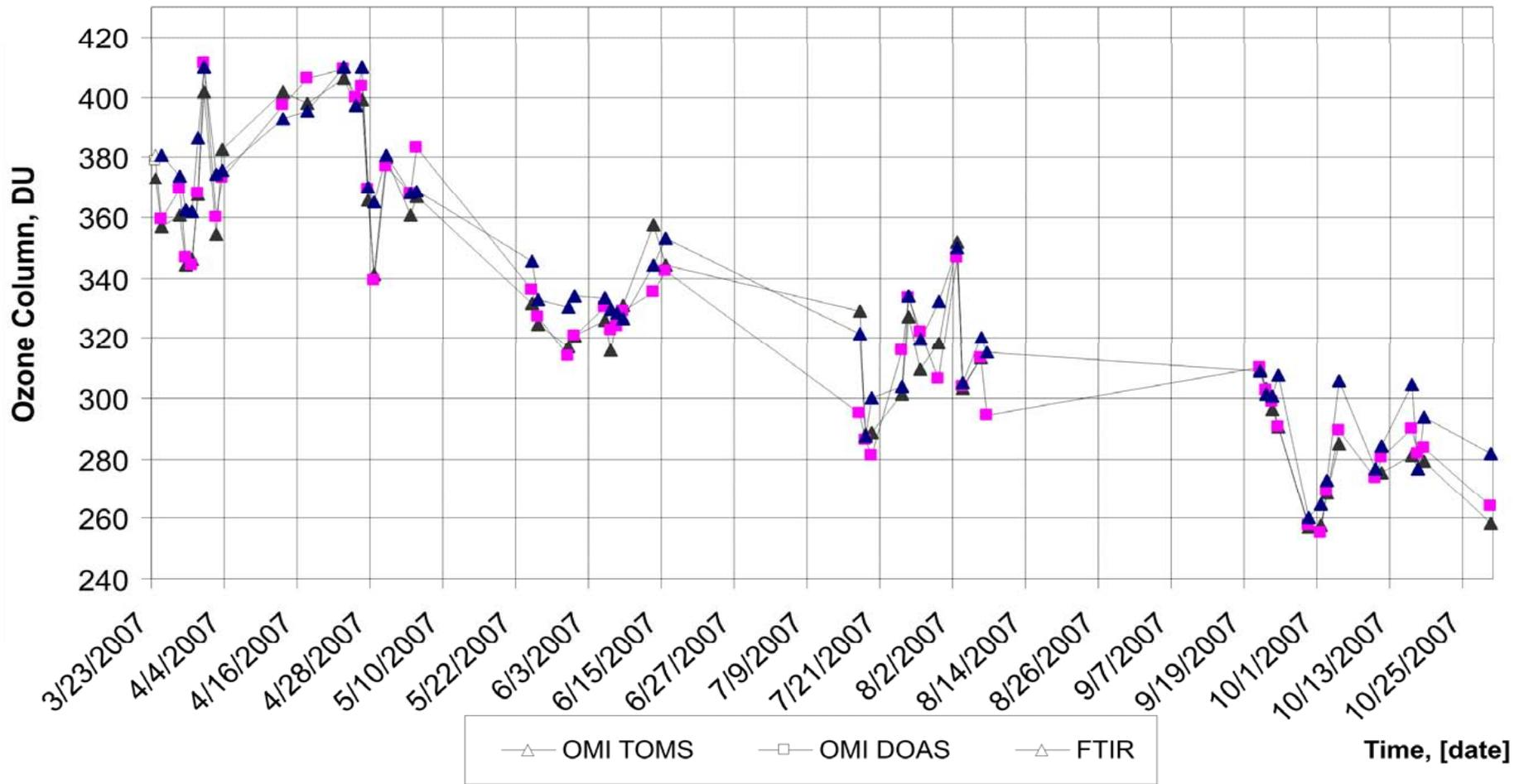
The total ozone column values retrieved from FTIR observations 2007 are biased low with respect to OMI-DOAS by  $-0.33$  DU and to OMI-TOMS by  $-4.33$  DU on average, where they have a relatively small standard error of about 1.4 %.
