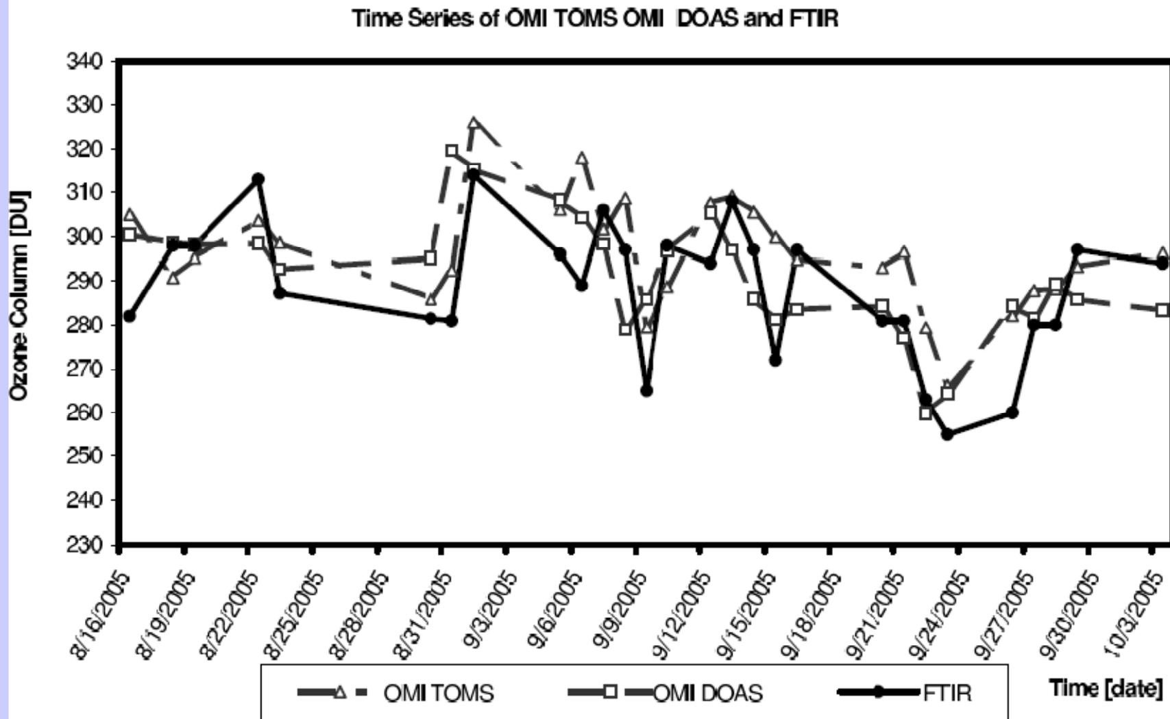
**Figure 4a: Time series of OMI total ozone (OMI-TOMS and OMI-DOAS) and ground based FTIR total ozone data for 2005. Average difference of satellite minus ground based amounts to 8.45 DU and 3.19 DU for OMI-DOAS and OMI-TOMS respectively, with a 10.50 DU and 13.41 DU standard deviation (1.98 DU and 2.53 DU standard errors).**
